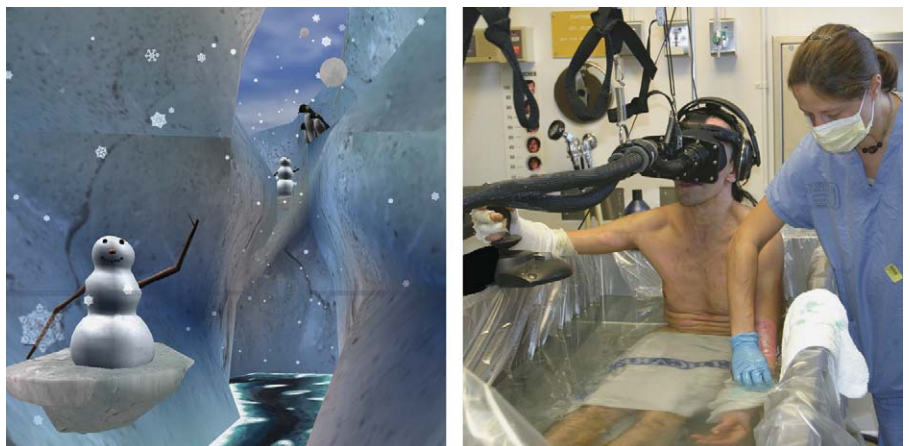
FIGURE 1. Right image: an adult burn patient using the water-friendly fiber-optic VR helmet to escape into SnowWorld pain distraction (shown on left) during wound debridement in the hydrotank. Instead of using electrons (electricity) the water-friendly helmet delivers photons (light) to the patient through the large black cables. Image on left by Ari Hollander, www.Imprintit.com , copyright, Hunter Hoffman, UW. Photograph on right, and copyright Hunter Hoffman, UW.
